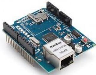
*Figura 7: Ethernet Shield W5100 WizNet*
